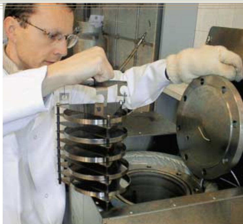
Test de vieillissement PAV (Pressure Ageing Vessel)
